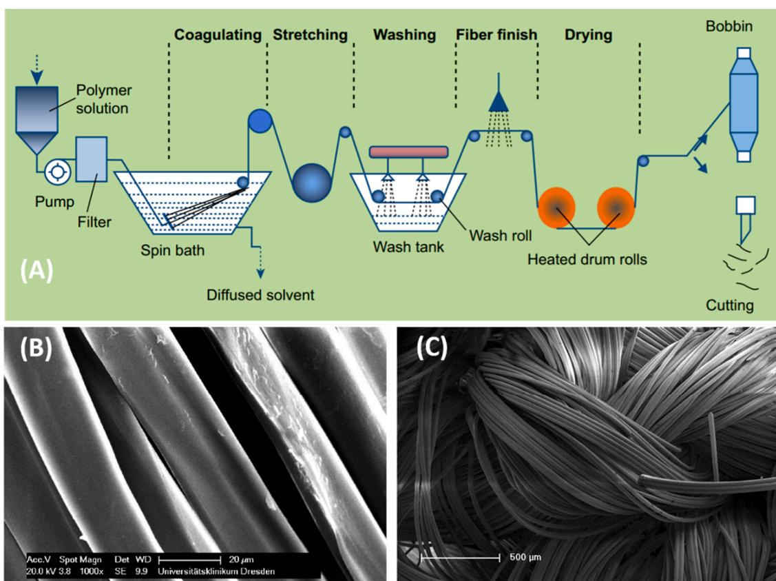
**Figure 3.** (A) Schematic illustration of the wet spinning process for yarn preparation adopted from [74]. (B) Chitosan microfibrers wet spun from an 8.5 wt% solution. (C) The constructed knitted fabric. Reprinted with permission from [75], copyright 2014 Taylor & Francis.
