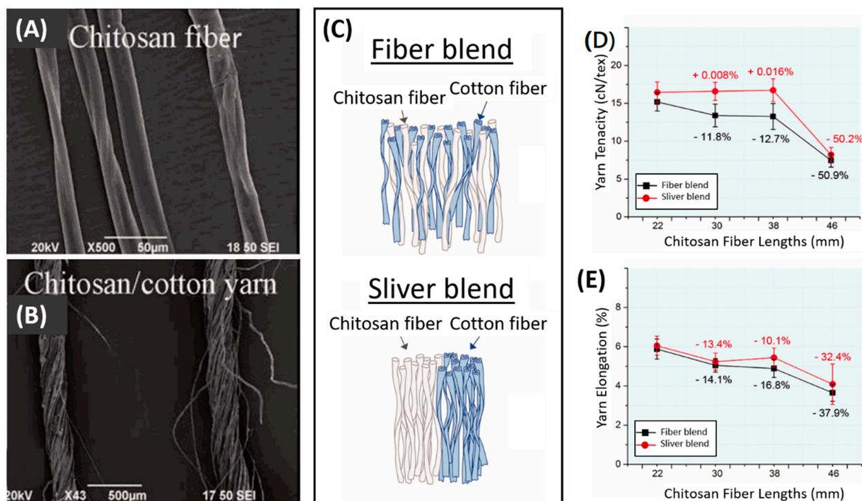
**Figure 4.** Micrograph images of surface structures in (A) chitosan fiber and (B) chitosan/cotton yarn. (C) Illustration of the blending methods. The yarn fiber blend showed higher (D) tenacity and (E) elongation than the yarn sliver blend at all chitosan fiber lengths. Reprinted with permission from [80,81], copyright 2014 & 2017 SAGE Publications.
