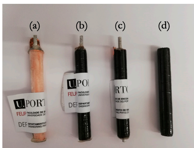
Figure 4. Showcase of the type of coaxial cells and parts investigated; (a) structural battery with thin glass fiber shell such as schematized in Figure 2a; (b) and (c) two coaxial cells that were analysed in this study; (d) CFRP shell.
