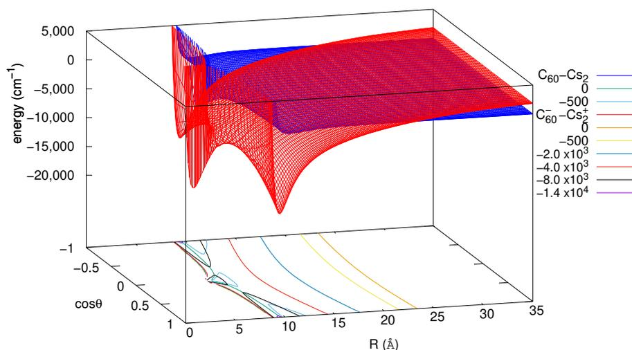
**Figure 2.** Analytic potential energy surfaces characterizing neutral  $\text{Cs}_2\text{-C}_{60}$  and ionic  $\text{Cs}_2^+\text{-C}_{60}^-$  pair interactions as a function of their relative distance  $R$  and orientation  $\theta$ .
