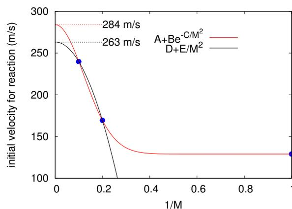
**Figure 12.** Extrapolation of initial velocity allowing for electron hopping to  $M \rightarrow \infty$ .
