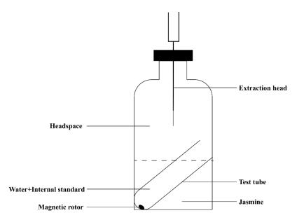
Figure 10. Diagram of aroma extraction device.
