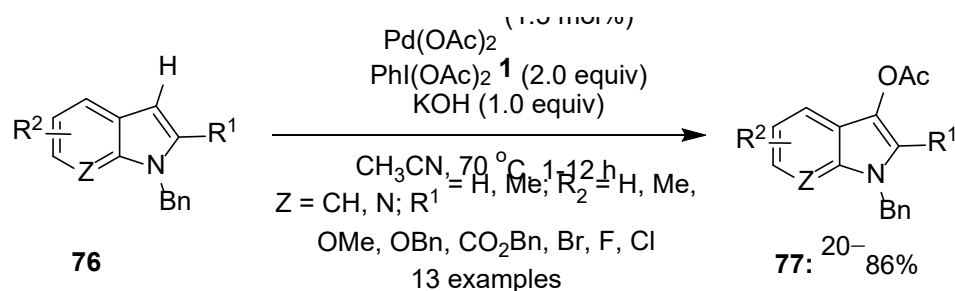
Scheme 23. Pd(II)-catalyzed C3-acetoxylation of substituted indoles 76 to afford C3-acetoxylated indoles 77 using \text{PhI}(\text{OAc})_2 1 .
