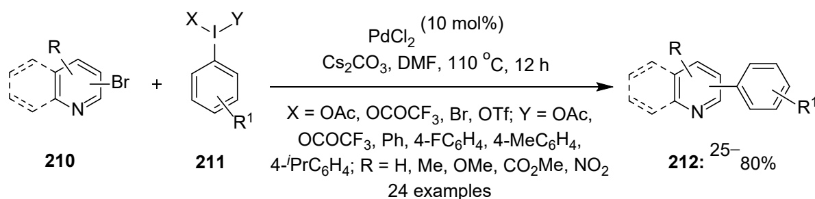
Scheme 66. Pd(II)-catalyzed arylation of N-heteroaromatic bromides 210 to access arylated heteroaromatic compounds 212 using hypervalent iodine(III) reagents 211 .
