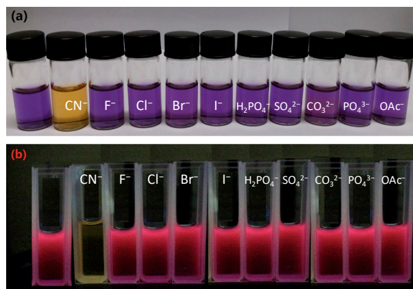
Figure 3. Cyanide ion detection with 509: (a) optically with the naked eye; (b) by fluorescence changes. Reproduced with permission from Wang et Al [359].
