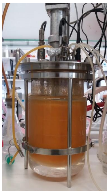
Figure 2. Phenazine production on a bioreactor cultivation of Pseudomonas chlororaphis subsp. aurantiaca DSM 19603.
