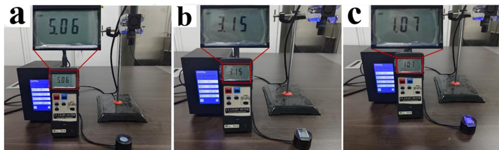
Figure 20. UV-shielding test: (a) blank sample; (b) B2 sample; and (c) C2 sample.
