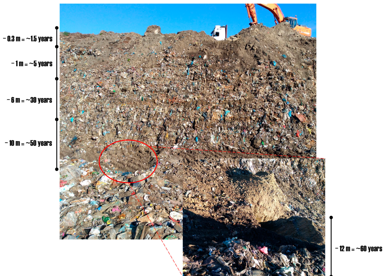
Figure 5. This schema illustrates the collection of soil samples from the municipal waste landfill (MWL), including the bottom layer of the pit (indicated by a red ring), which corresponds to various (bio)degradation periods.
