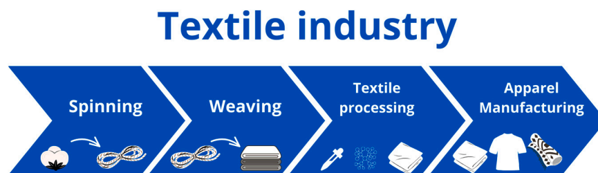
Figure 1. The flow chart of the textile manufacturing process.
