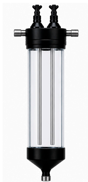
Figure 10. Schematic configuration of the membrane-less flow-by tubular alkaline electrolyzer used in the experiments.
