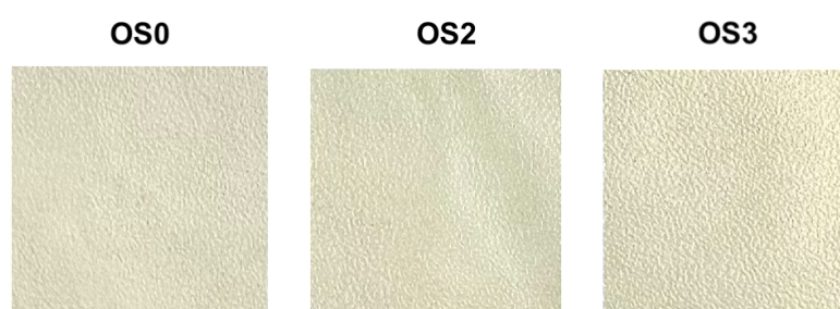
Figure 1. Macroscopic appearance of solution-cast chitosan-alginate films: OS0 (control), OS2 (turmeric-enriched), and OS3 (oregano-enriched).
