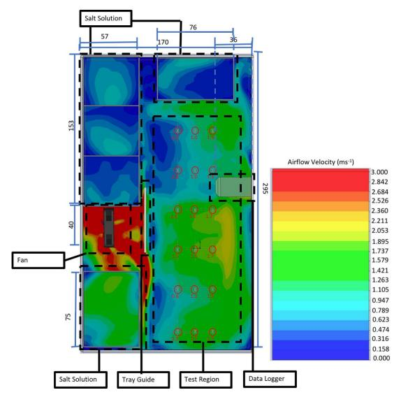
**Figure 1.** Schematic of test chamber 2 with a cut point of 1 mm above sample plane. All measurements on the outside of the box are in mm. Each area of the chamber is highlighted with a dotted line. Eighteen inoculum droplets can be placed on nonporous surface samples and placed within the test region. Numbers underneath the sample locations indicate airspeed (ms<sup>-1</sup>). Colour overlay represents airflow (ms<sup>-1</sup>), with colours corresponding to the key to the right.
