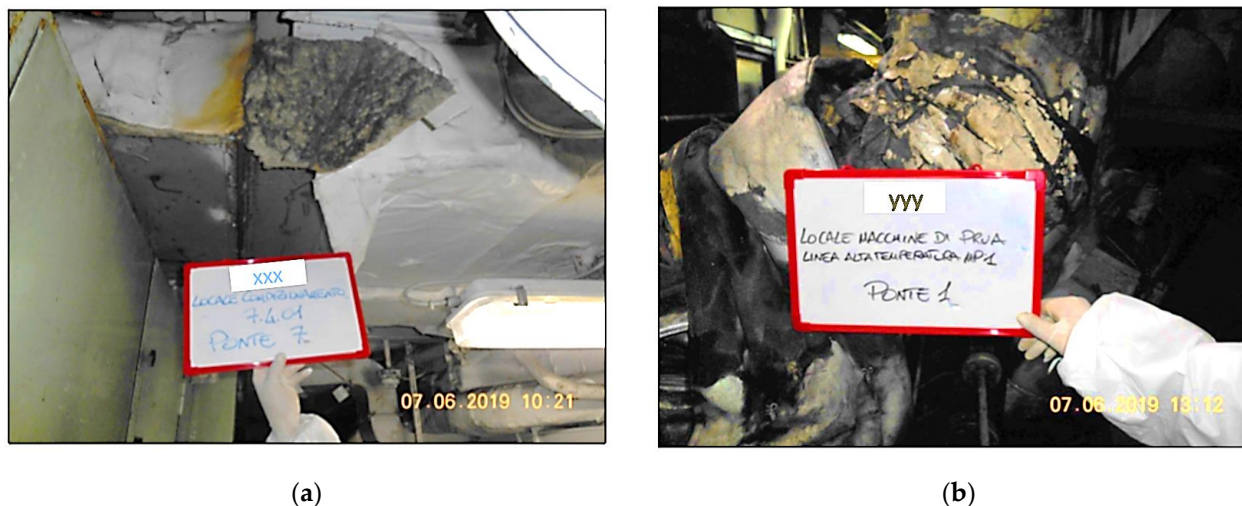
Figure 1. Examples of pictures taken during mass sampling on board ships: (a) MMFVs H351, sampled in “air conditioning room 7.4.01 Deck n. 7”. (b) MMFVsNSC, sampled in “bow engine room—high temperature line P1 Deck 1”.
