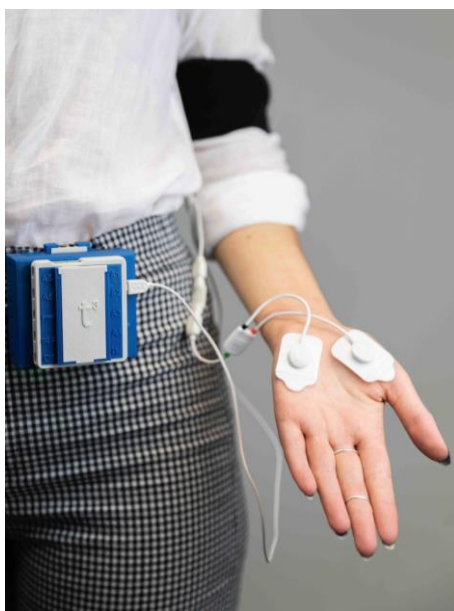
Figure 4. The electrodermal activity (EDA) device. The electrodes on the hand are connected to sensor cables which are connected to the portable EDA device. A black armband is on the arm to secure the sensor cable.
