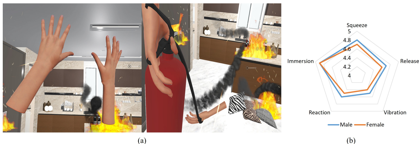
Figure 13. Training the use of a fire extinguisher using the haptic glove: (a) VR application and (b) radar chart (force feedback for squeezing and releasing the handle, nozzle vibration and reaction, and VR immersion) surveyed from user experiences.
