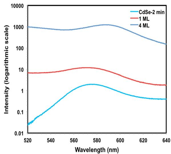
**Figure S2.** The PL spectrum of CdSe two-minute aliquot QDs and the core-shell CdSe-ZnO with 1 and 4 MLs of ZnO.
