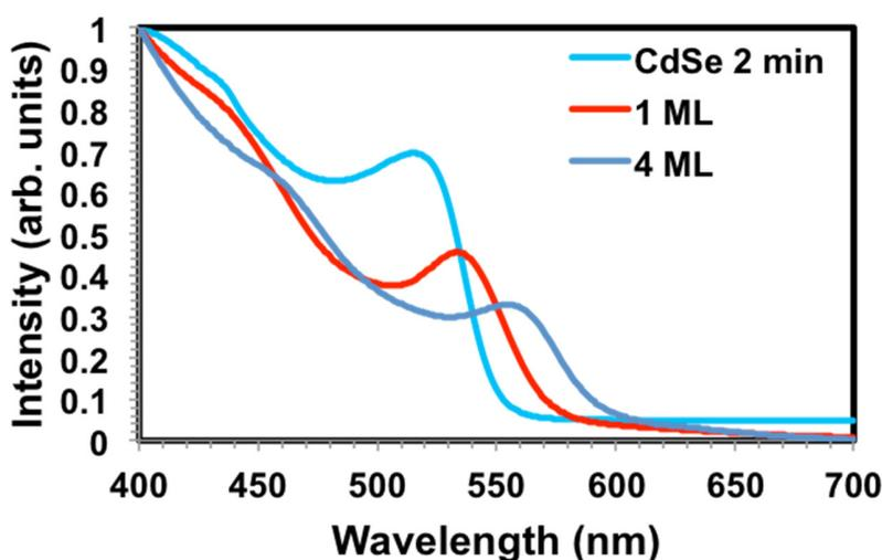
**Figure S1.** The absorption spectrum of CdSe two-minute aliquot QDs and the core-shell CdSe-ZnO with 4 MLs of ZnO.
