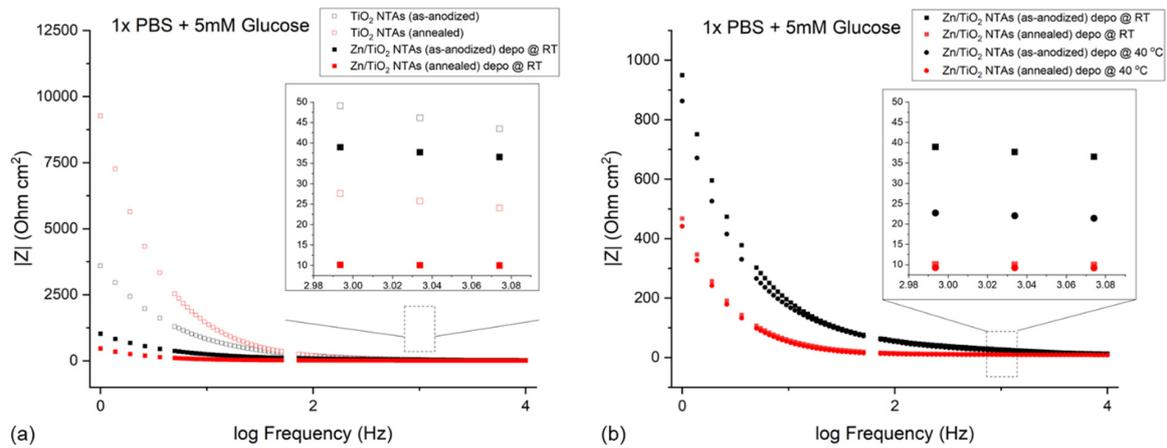
**Figure 6.** (a) Normalized impedance spectra of Zn/TiO<sub>2</sub> NTA samples tested in a pure 1X PBS solution with 5 mM glucose compared to reference TiO<sub>2</sub> NTAs. (b) Normalized impedance spectra of Zn/TiO<sub>2</sub> NTA samples deposited under different temperatures tested in a pure 1X PBS solution with 5 mM glucose.
