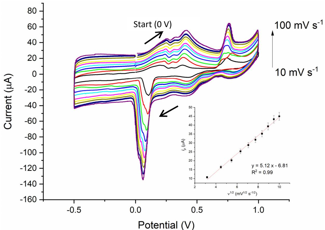
**Figure 3.** CV of Zn/TiO<sub>2</sub> NTAs in a 0.1 M NaOH solution with 5 mM of glucose in scan rates from 10  $\text{mV s}^{-1}$  to 100  $\text{mV s}^{-1}$ . Different colors are used to differentiate varying scan rates. The inset is the current peak vs. square root of scan rate, and the red dash line is for an eye guide only.
