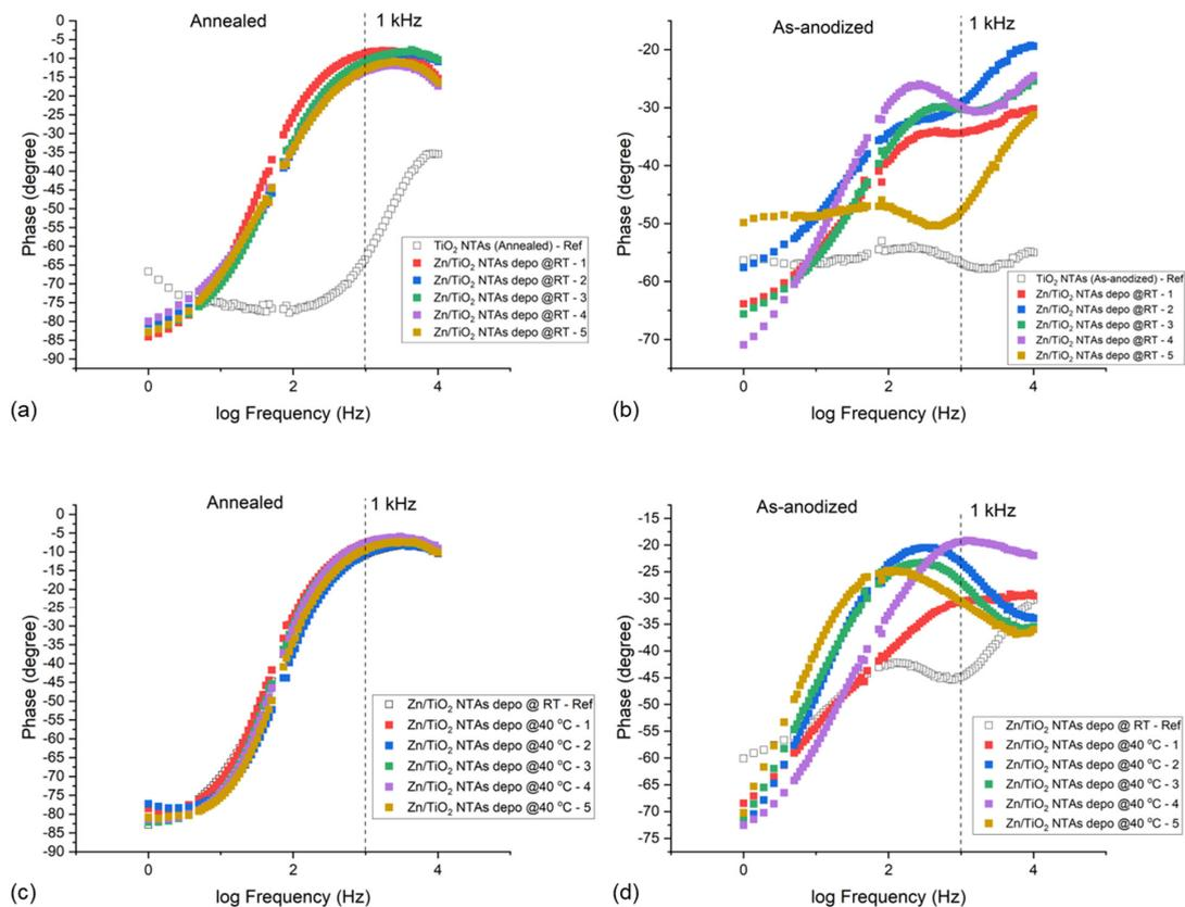
**Figure 7.** Phase plots for (a) Zn/TiO<sub>2</sub> NTAs (annealed), (b) Zn/TiO<sub>2</sub> NTAs (as-anodized) with zinc deposited at room temperature, (c) Zn/TiO<sub>2</sub> NTAs (annealed), and (d) Zn/TiO<sub>2</sub> NTAs (as-anodized) with zinc deposited at 40 °C. EIS was performed in a pure 1X PBS solution + 5 mM glucose.
