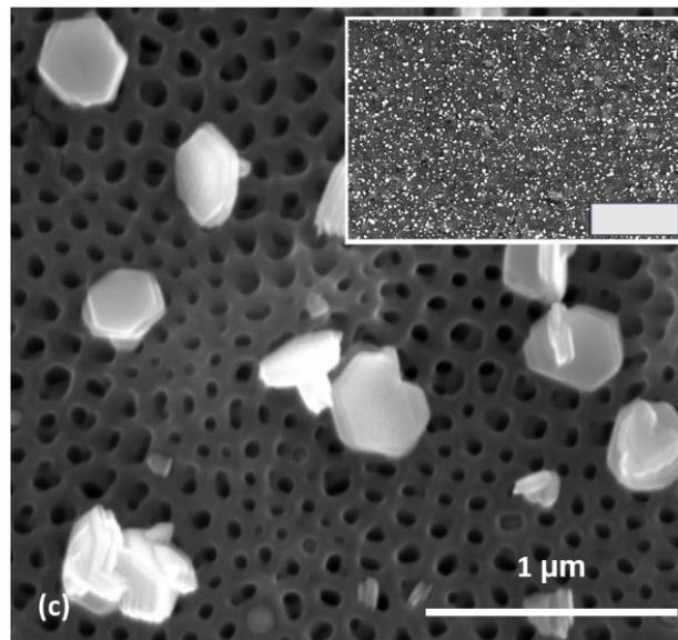
**Figure 1.** Top-view SEM images of (a) annealed TiO<sub>2</sub> NTAs with the inset showing the cross section, (b) Zn/TiO<sub>2</sub> NTAs (annealed) deposited at room temperature, and (c) Zn/TiO<sub>2</sub> NTAs (annealed) deposited at 40 °C. The scale bars in the insets show (a) 2 μm, (b) 10 μm, and (c) 10 μm, respectively.
