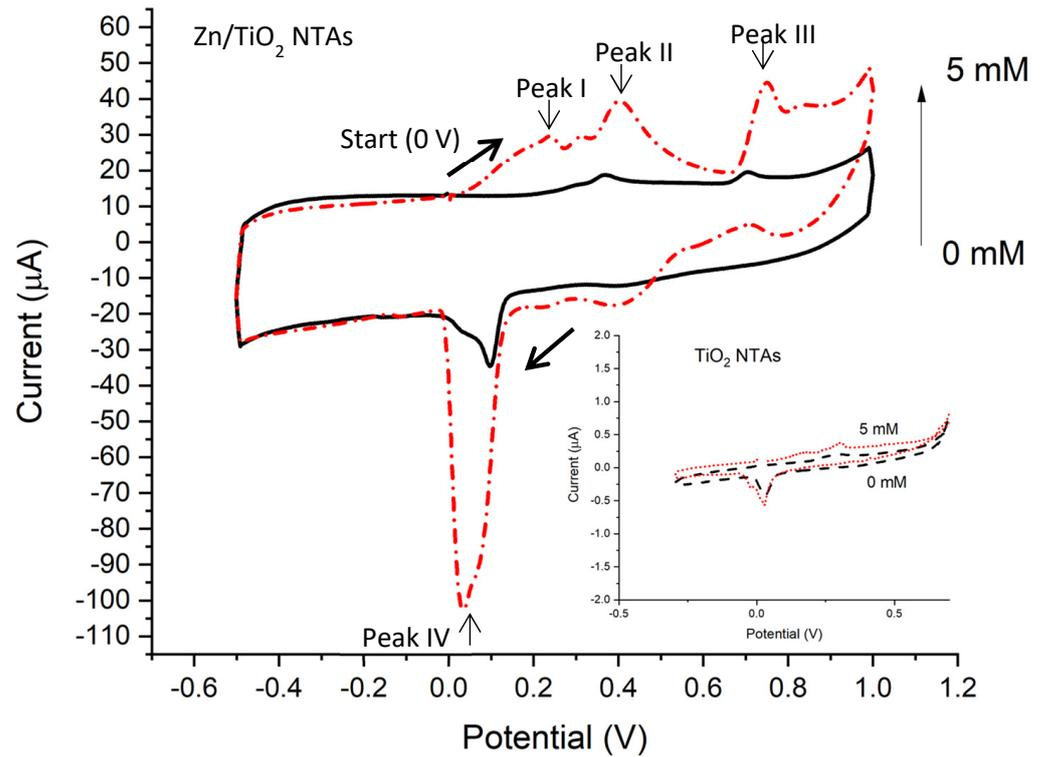
**Figure 4.** CV of TiO<sub>2</sub> NTAs (inset) and Zn/TiO<sub>2</sub> NTAs in a 0.1 M NaOH solution containing 0 mM and 5 mM of glucose (at a scan rate of 50 mV s<sup>-1</sup>). The red dashed curve refers to 5 mM glucose concentration, and the black solid curve refers to 0 mM glucose concentration. The arrows indicate potential sweep directions.
