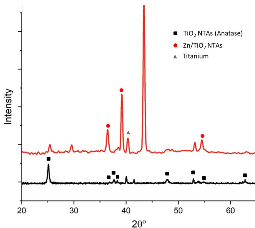
**Figure 2.** XRD patterns of 40 °C-deposited Zn/TiO<sub>2</sub> NTAs (annealed) reconstructed from our previous work [30], showing zinc peaks with peak positions (circles). The peak positions for TiO<sub>2</sub> (anatase) (squares) and for the titanium (triangle) are identified.
