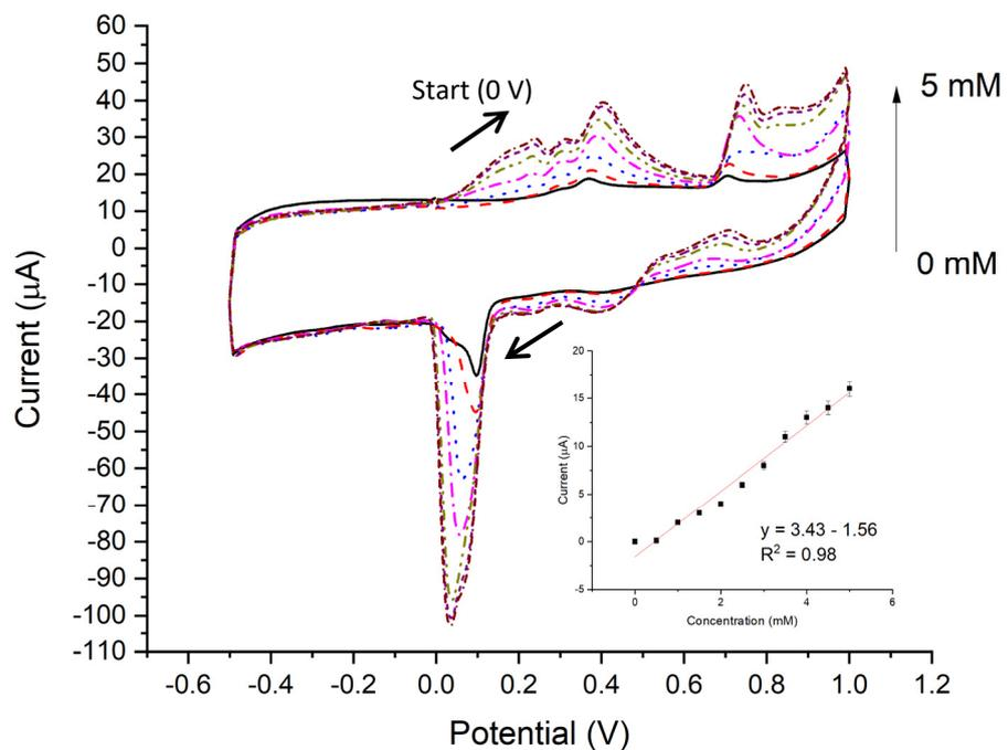
**Figure 5.** CV on Zn/TiO<sub>2</sub> NTAs in a 0.1 M NaOH solution with different glucose concentrations (at a scan rate of 50 mV s<sup>-1</sup>). Different colors of the curves refer to the varying glucose concentrations. The inset shows the calibration curve of the oxidation peak's current values. The legends describe glucose concentrations in the 0.1 M NaOH solution.
