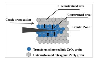
Figure 11. Schematic illustration of stress-induced phase transformation toughening.
