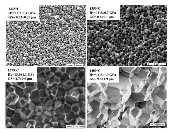
**Figure 6.** Field Emission Scanning Electron Microscopy (FESEM) micrographs of  $Y_3Al_5O_{12}$  (YAG) sintered by Spark Plasma Sintering (SPS) at increasing temperatures (Hv = average Vickers hardness; GS = average grain size) [41].
