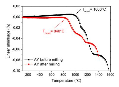
**Figure 4.** Linear shrinkage *versus* sintering temperature (during the heating step) of un-milled (black curve) and milled (red curves) AY powders. Maximum sintering temperatures were 1420 °C and 1600 °C for the milled and un-milled powders, respectively [34].
