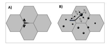
**Figure 9.** Schematic illustration of the residual stress field in (**a**) pure  $Al_2O_3$ , due to thermal expansion anisotropy during cooling and (**b**)  $Al_2O_3/SiC$  nanocomposites, due to thermal expansion coefficient mismatch between matrix and second-phase. In both figures, the preferential crack path is illustrated.
