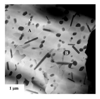
**Figure 14.** TEM micrograph of  $Zr_{0.89}Ce_{0.11}O_2/Al_2O_3/SrAl_{12}O_{19}$  composite, produced by the surface modification method. Letters A, B and C denote the Ceria-stabilized ZrO<sub>2</sub>, the  $\alpha$ -Al<sub>2</sub>O<sub>3</sub> and the SrAl\_{12}O\_{19} phases, respectively, as determined by EDX analysis.
