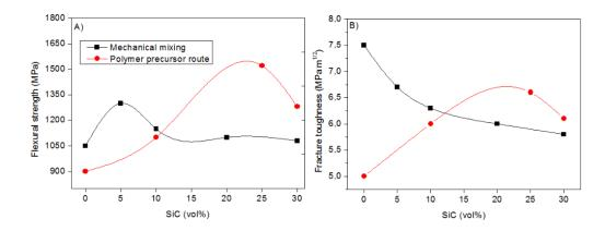
**Figure 12.** (a) Flexural strength and (b) fracture toughness of S<sub>3</sub>N<sub>4</sub>/SiC composite as a function of the SiC volume content. Black symbol: powder by conventional mixing and milling method [113]; red symbol: powder by polymer precursor route [114]. Redrafted from [71].
