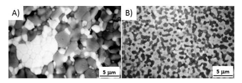
**Figure 13.** SEM micrographs of  $Al_2O_3/50_{vol.}$ %YAG sintered materials, prepared by (a) traditional mixing route and (b) co-precipitation, both sintered at 1600 °C for 3 h.
