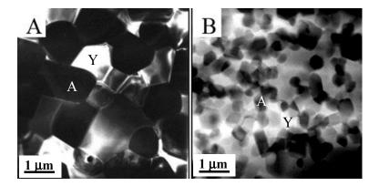
**Figure 5.** Transmission Electron Microscopy (TEM) images of AY materials. (**a**) Un-milled powder, sintered ad 1600 °C/3 h; (**b**) Milled powder sintered at 1420 °C/3 h. Characters A and Y refer to  $\alpha$ -Al<sub>2</sub>O<sub>3</sub> (black grains) and YAG (white grains), respectively.
