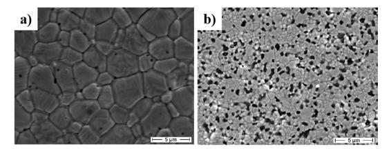
**Figure 7.** FESEM micrographs of (a) pure CeO<sub>2</sub>-stabilized ZrO<sub>2</sub> and (b) the respective composite containing  $16_{vol.}$ % of  $\alpha$ -Al<sub>2</sub>O<sub>3</sub>, both sintered at 1450 °C for 1h [70].
