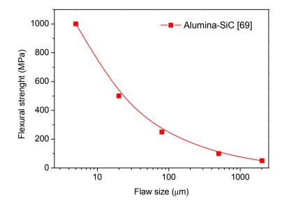
Figure 8. Evolution of flexural strength with the flaw size in Al<sub>2</sub>O<sub>3</sub>/SiC composites [69].
