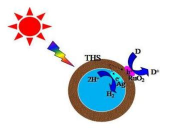
Scheme 2. The photocatalytic hydrogen production on Ag-I-RuO<sub>2</sub>-O-THS.
