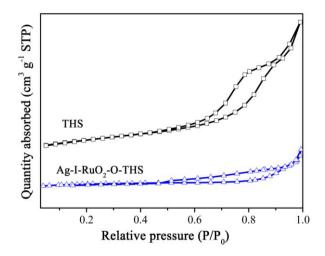
Figure 2. N<sub>2</sub> adsorption-desorption isotherms of THS and Ag-I-RuO<sub>2</sub>-O-THS.
