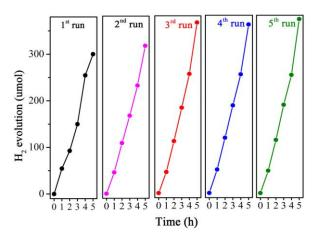
Figure 7. Stability of Ag-I-RuO<sub>2</sub>-O-THS during prolonged photocatalytic operation.
