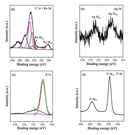
**Figure 4.** X-ray photoelectron spectroscopy (XPS) spectra of Ag-I-RuO<sub>2</sub>-O-THS: (**a**) C 1s and Ru 3d; (**b**) Ag 3d; (**c**) O 1s; (**d**) Ti 2p.
