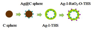
**Scheme 1.** Processes involved in the formation of dual cocatalysts co-loading on the TiO<sub>2</sub> hollow spheres (THS).
