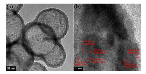
**Figure 3.** (**a**) Transmission electron microscopy (TEM) and (**b**) High resolution transmission electron microscopy (HRTEM) images of Ag-I-RuO<sub>2</sub>-O-THS.
