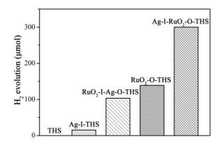
**Figure 6.** Photocatalytic activities of H<sub>2</sub> evolution on THS loaded by the cocatalysts with different spatial dispersion.
