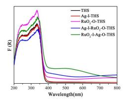
**Figure 5.** Ultraviolet-visible diffuse reflectance spectra (UV-Vis DRS) of THS loaded by the cocatalysts with different spatial dispersion.
