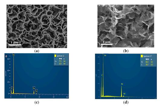
**Figure 2.** (**a**,**b**). Representative SEM images of graphene nanowalls produced from (**a**) methane on copper substrate and (**b**) from bagasse on nickel substrate. (**c**,**d**) EDS spectra of graphene formed from (**c**) methane on copper substrate and (**d**) from bagasse on nickel substrate.
