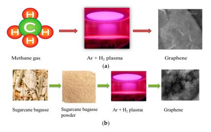
**Figure 6.** Schematic representation of plasma enabled synthesis of graphene. (**a**) Conversion of methane gas into graphene in the presence of plasma. (**b**) Reforming of sugarcane bagasse into graphene.
