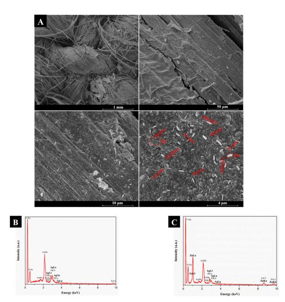
**Figure 4.** FESEM images of flax fabric functionalized with both AgNPs and ZnONPs (**A**). Magnifications of 1 mm, 50  $\mu$ m, 10  $\mu$ m, and 4  $\mu$ m (from the left to the right). EDS spectra of Z1 zone (**B**) and Z2 zone (**C**).
