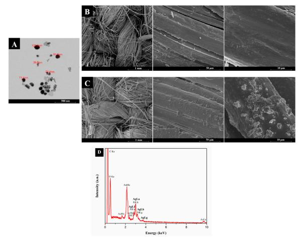
**Figure 3.** Scanning transmission electron detector (STEM) micrograph of the AgNPs synthesized in polyethylene glycol (PEG) solution with magnifications of 500 nm (**A**). Field Emission Scanning Electron Microscopy (FESEM) images of untreated flax (**B**) and flax + AgNPs (**C**) with magnifications of 1 mm, 50  $\mu$ m and 10  $\mu$ m (from the left to the right). The images are in topographic mode. Energy Dispersive Spectroscopy (EDS) spectrum of flax fabric treated with AgNPs (**D**).
