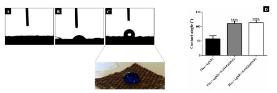
**Figure 10.** Representative images of water contact angle (WCA) of untreated flax (**A**), flax + AgNPs (**B**) and flax + AgNPs + 0.4 MZnONPs (**C**). Comparison between the WCA values (**D**). Values are represented by mean  $\pm$  SD. Flax + AgNPs vs. flax + AgNPs + ZnONPs: \*\*\*\*: *p* < 0.0001.
