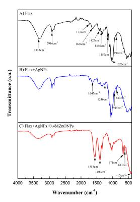
**Figure 6.** Attenuated Total Reflectance-Fourier Transform Infrared Spectroscopy (ATR-FTIR) spectra of flax fabric (**A**), flax functionalized with AgNPs (**B**), and flax functionalized with AgNPs and ZnONPs (**C**).
