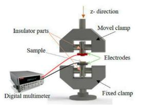
**Figure 1.** Schematic representation of the experimental configuration of the clamps for the compression experiments with simultaneous electrical measurements for electro-mechanical response evaluation of the samples.
