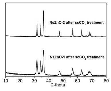
Figure 4. XRD patterns of NsZnO-1 and NsZnO-2 after scCO<sub>2</sub> treatment.
