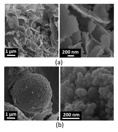
Figure 2. FESEM images of nanostructured (Ns)ZnO-1 (a) and NsZnO-2 (b).
