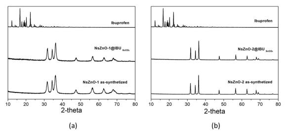
**Figure 5.** (a) XRD patterns of NsZnO-1, IBU@NsZnO-1, and pure crystalline IBU. (b) XRD patterns of NsZnO-2, IBU@NsZnO-2, and pure crystalline IBU.
