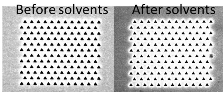
**Figure S9.** SEM images showing the surface before and after exposure to the solution. There is no corruption or distortion to the structures, nor is there any peeling of the gold film.
