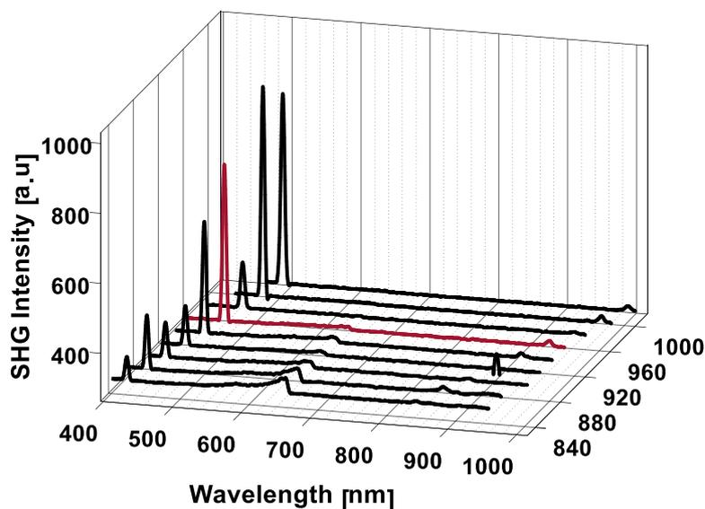
**Figure S6.** SHG at different fundamental WL varying from 840 to 1000nm with 20nm intervals. Some filters were removed allowing the appearance of some fluorescence and fundamental beam residues. When scanning the SHG intensity plots these filters were placed in the beam path and removed these residues.
