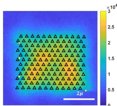
**Figure S2.** SHG intensity map of the structure used coated by a thin layer ( $\sim 150\text{nm}$ ) of PVA. The triangles are overlaid to guide the eye.
