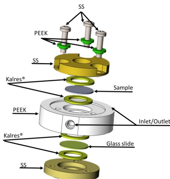
**Figure S1.** Blown up scheme of cell used showing the different elements used and their chemical components.
