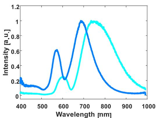
**Figure S8.** Transmission spectra of the structure with PVA coating – light blue, and immersed in DME – blue line. The plasmon modes are at 748 and 600nm for the PVA coating, and 569 and 690nm for DME. Showing no resonance with the fundamental wavelength used.
