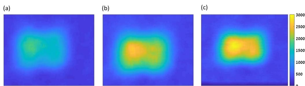
**Figure S3.** Comparison of structure with different environments. Scaled to the same intensity. A hexagonal array of equilateral triangles with a side length of  $200\text{nm}$  and a center-to-center distance of  $400\text{nm}$ . Scans were taken in (a) DME, (b) DME after exposure to ambient conditions, and (c) DME/ $\text{H}_2\text{O}$   $0.33\text{M}$ .
