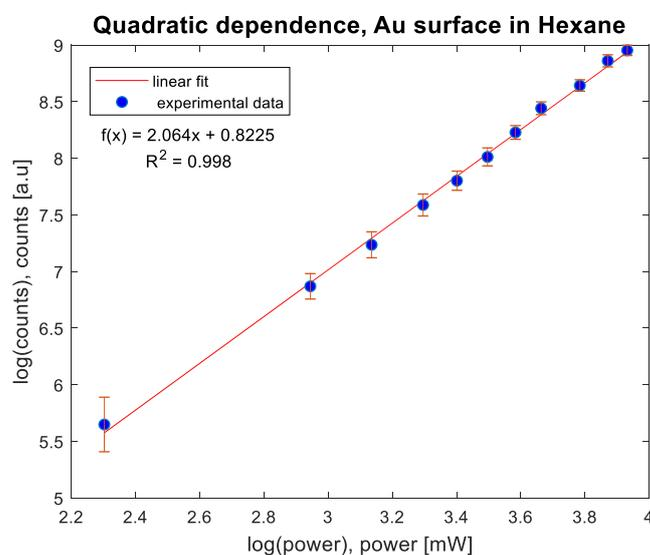
**Figure S5.** log-log plot of SHG signal versus laser intensity power. The slope is approximately 2 with an  $R^2$  value larger than 0.99, showing that indeed SHG is collected.
