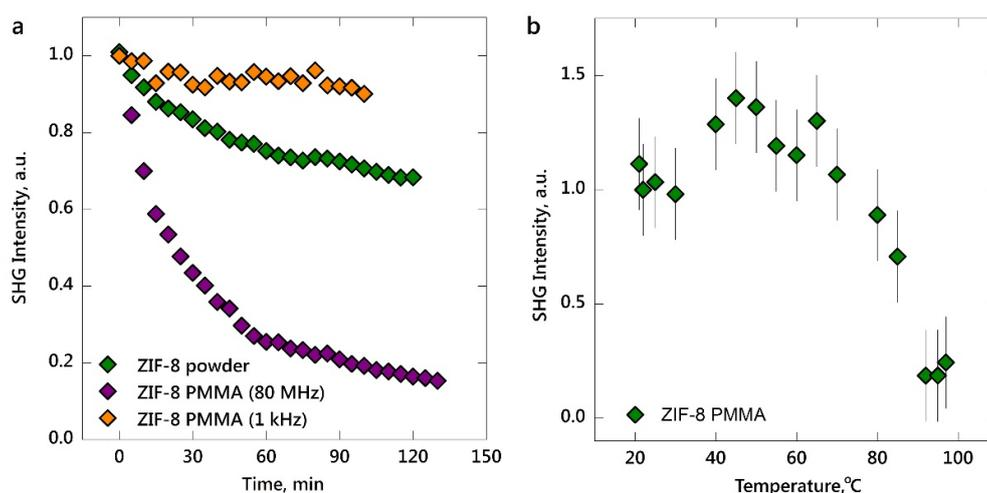
**Figure 3.** (a) Evolution of the SHG intensity for ZIF-8 powder and ZIF-8–PMMA composite upon laser radiation (1047 nm central wavelength, 150 fs pulse duration, 80 MHz and 1 kHz repetition rate) with an integral power of 100 mW (80 MHz) and 10 mW (1 kHz). (b) The thermal stability of SHG signal, excited by 50 mW at an 80 MHz repetition rate, for the ZIF-8–PMMA composite analyzed by heating on the Peltier element.
