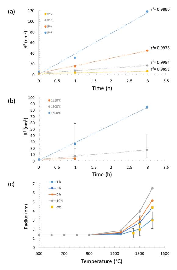
**Figure 9.** Ostwald ripening of the nano-oxides: (a) evolution of the radius elevated at the power p (p = 2, 3, 4, 5) against time for a thermal annealing at 1300 °C; (b) evolution of the cube radius against time for thermal annealing at 1250 °C, 1300 °C and 1400 °C; (c) plot of the calculated and experimental radii against temperature for various annealing durations.
