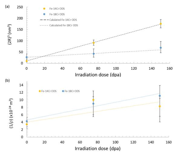
**Figure 13.** Radius and density evolution after 0, 75 and 150 dpa in both Fe-14Cr ODS and Fe-18Cr ODS: (a) evolution of the cube diameter against irradiation damage, (b) evolution of the inverse of the density against irradiation damage.
