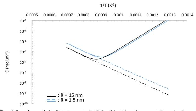
**Figure 2.** Dependence on the irradiation temperature irradiation of the yttrium solute concentration produced by recoil resolution and by thermal solubility for pyrochlore-type precipitate.
