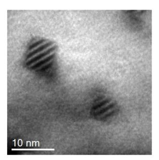
**Figure 8.** TEM image of two cubical pyrochlore oxides after coarsening at 1300 °C.
