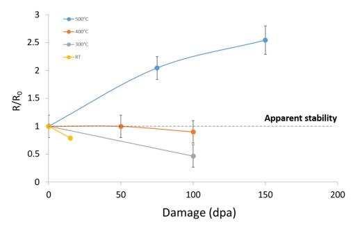
**Figure 14.** Evolution of the nano-oxides' normalized radii after irradiation at RT,  $300 \,^{\circ}\text{C}$ ,  $400 \,^{\circ}\text{C}$  and  $500 \,^{\circ}\text{C}$ .
