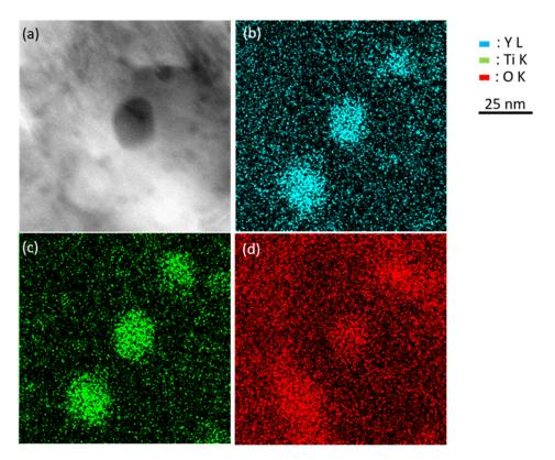
**Figure 4.** Chemical map of the nano-oxides from EDS acquisition: (a) ADF STEM image, (b) Y L ac-quisition, (c) Ti K acquisition, and (d) O K acquisition.
