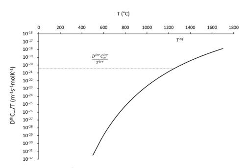
**Figure 15.** Evolution of  $\frac{D^{th}C_{\infty}}{T}$  against temperature, used in order to determine the equivalent temperature.
