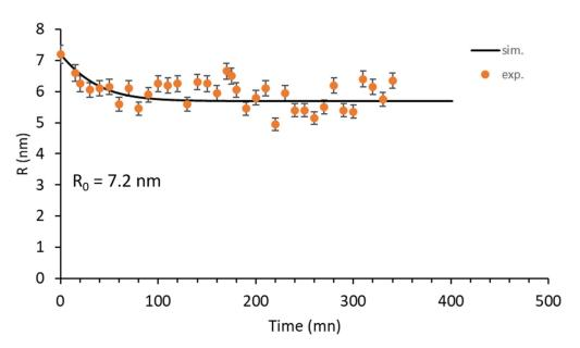
**Figure 11.** Experimental and theoretical dissolution rate of the nano-oxide presented in Figure 9 during in situ  $4 \text{ MeV Au}^{2+}$  ion irradiation.
