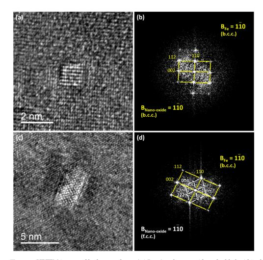
**Figure 6.** HRTEM images of both nano-cluster (<1.5 nm) and nano-oxide embedded within the ferritic matrix: (a) HRTEM image of a nano-cluster, (b) corresponding FFT, (c) HRTEM image of a nano-oxide, (d) corresponding FFT.
