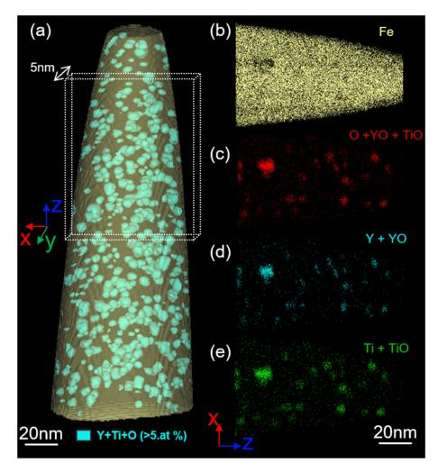
**Figure 5.** Three-dimensional APT reconstruction of as-received Fe-14Cr ODS: (a) an iso-composition surface >5 at.% of O+Y+Ti in blue was used to highlight nano-oxides, (b–e) zoomed in insert of region of interest showing map of Fe, O, Y and Ti atoms in as-received Fe-14Cr ODS steel.
