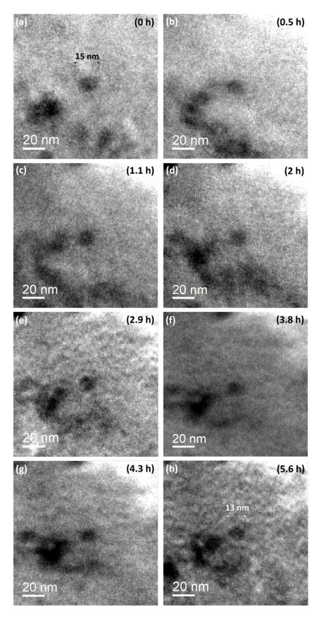
**Figure 10.** In situ observation of the evolution of a nano-oxide during 4 MeV  $Au^{2+}$  irradiation: (a) before irradiation, (b) after 0.5 h (1.3 dpa), (c) after 1.1 h (3 dpa), (d) after 2 h (5 dpa), (e) after 2.9 h (8 dpa), (f) after 3.8 h (10 dpa), (g) after 4.3 h (12 dpa), and (h) after 5.6 h (15 dpa).
