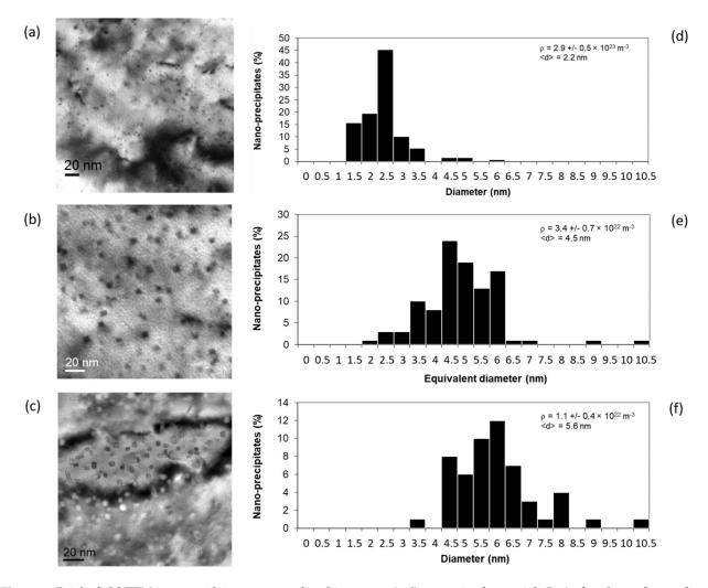
**Figure 3.** Bright field TEM image with its corresponding histogram: (**a**,**d**) as-received material, (**b**,**e**) after thermal annealing (1300  $^{\circ}$ C, 1 h), (**c**,**f**) after irradiation up to 150 dpa at 500  $^{\circ}$ C.
