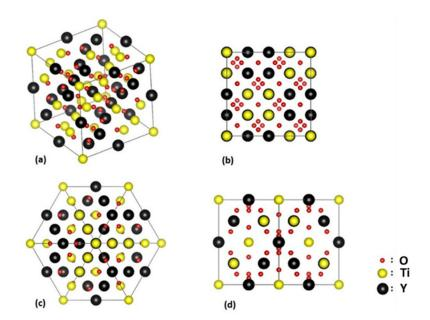
**Figure 7.** Pyrochlore-type lattice structure: (a) general view, (b) observed along the (001) direction, (c) observed along the (111) direction, (d) observed along the (011) direction.
