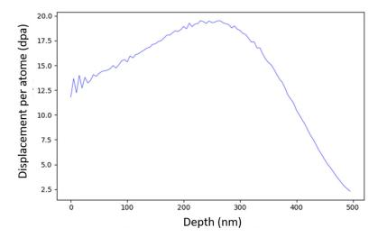
**Figure 1.** Depth profile of irradiation damages (displacement per atom) in Fe calculated by Iradina [14] using  $4000 \text{ keV-Au}^{2+}$  ions with a fluence of  $4.0 \times 10^{15} \text{ ions} \cdot \text{cm}^{-2}$ .
