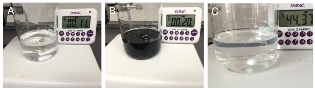
Figure 2. Photographs of the experimental process of Bi(NO 3 ) 3 reduction with NH 3 BH 3 without rGO support. (A) Bi(NO 3 ) 3 solution in the ethylene glycol, (B) NH 3 BH 3 added in the solution, (C) Continuous stirring for approximately 45 min.
