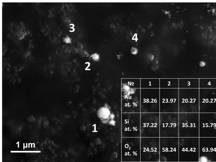
**Figure 3.** High-angle annular dark field (HAADF) SEM image of hybrid NPs obtained from 30/180 nm Au/Si film and transferred to carbon tape. Legend shows corresponding contents of gold and silicon in atomic percents found by EDX at positions marked by numbers 1–4.
