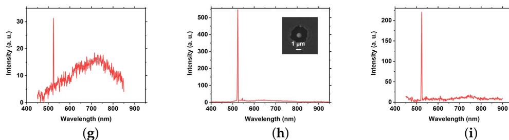
**Figure 4.** PL measurements of single hybrid NP obtained from bi-layer Au/Si films with different thickness ((a,d) 10/100 nm, (b,e) 30/180 nm and (c,f) 30/90 nm: (a–c) PL spectra; (d–f) dependencies of broadband PL intensity on pump fluence; PL spectra of initial bi-layer Au/Si (30/180 nm) film (g), single gold (h) and silicon (i) NPs. Insets show corresponding SEM images of single NPs.
