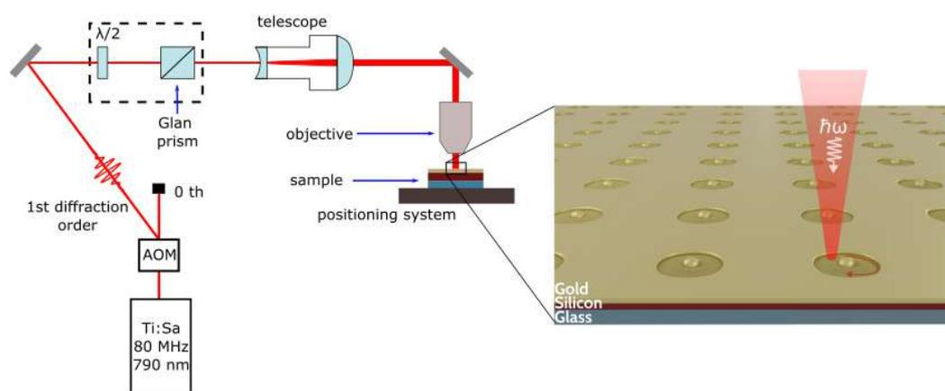
**Figure 1.** Schematic illustration of experimental setup used for particle fabrication. Inset illustrates a formation of hybrid nanoparticles array under femtosecond laser cutting of patch from a Au/Si bi-layer film on a glass substrate.
