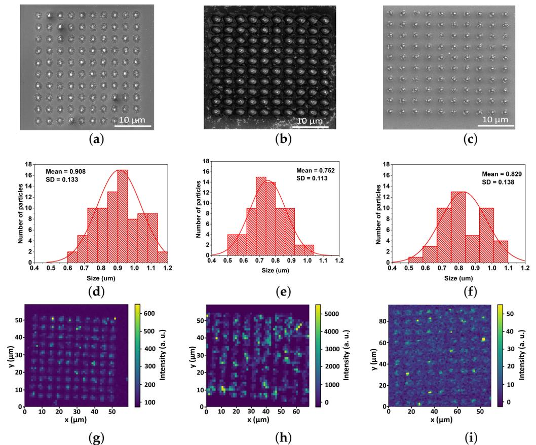
**Figure 2.** Arrays of hybrid NPs obtained from bi-layer Au/Si films with different thickness (first column—10/100 nm, second column—30/180 nm and third column—30/90 nm): (a–c) SEM images; (d–f) size distribution histograms with a mean size (mean) and the standard deviation of the size (SD); (g–i) PL signal mapping, brighter areas correspond to higher intensity at 600 nm wavelength.
