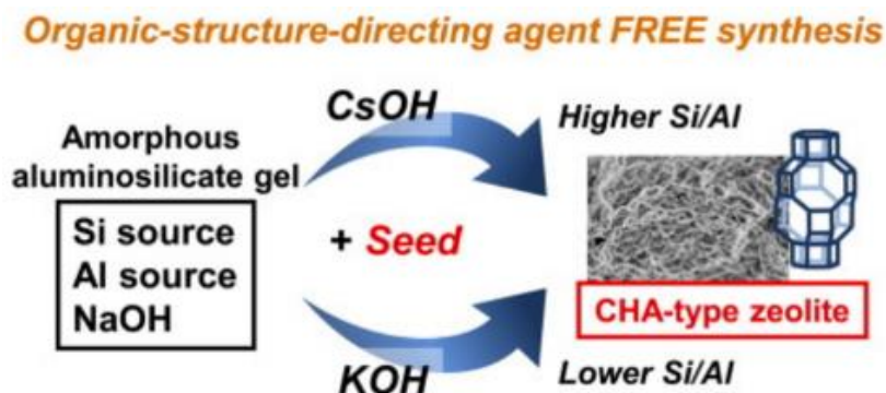
Figure 2. Schematic diagram of the CHA zeolite by a seed-assisted method in the absence of organic structure-directing agents. Reprinted with permission from ref. [40]. Copyright 2014, Elsevier.
