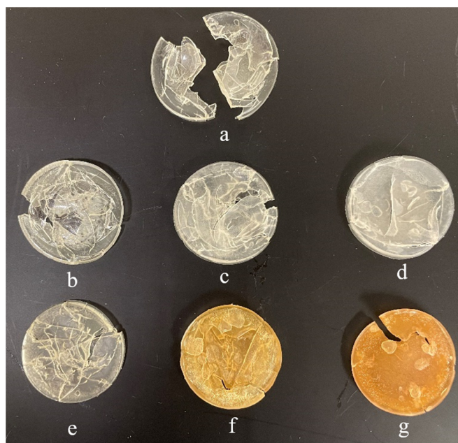
Figure 6. Dried gels after pulsatile swelling: (a) FC34, (b) 0.1NCB_FC34, (c) 1.0NCB_FC34, (d) 3.0NCB_FC34, (e) 0.1NCSM_FC34, (f) 1.0NCSM_FC34, and (g) 3.0NCSM_FC34.
