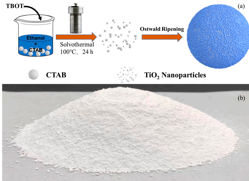
Figure 1. (a) Illustration of the preparation of TiO 2 -100; (b) The nanoporous TiO 2 -100 were synthesized on a scale of 5 times.
