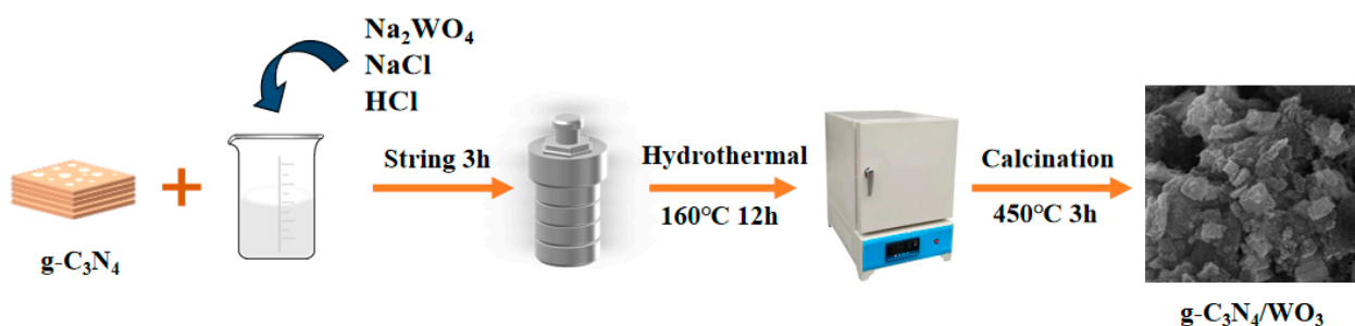
Scheme 1. Schematic diagram of the preparation of g-C 3 N 4 /WO 3 .
