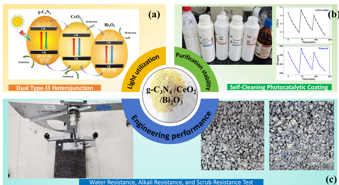
Figure 1. Schematic of g\text{-C}_3\text{N}_4/\text{CeO}_2/\text{Bi}_2\text{O}_3 dual type-II heterojunction photocatalysis self-cleaning coatings: (a) dual type-II heterojunction structure design; (b) purification based on self-cleaning coatings; (c) engineering performance under real road condition.
