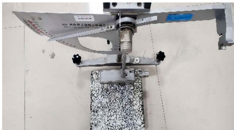
Figure 17. Pendulum instrument measures the pendulum value of self-cleaning coating.
