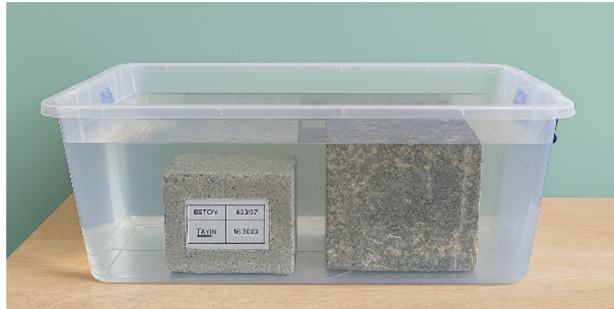
Figure 5. Concrete specimens immersed in water.
