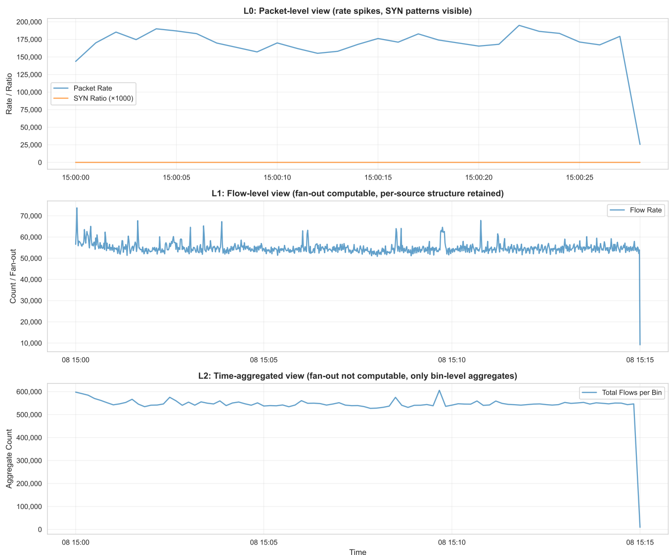
Figure 6. Trace of port-scan-like behavior across evidence layers. L0 shows packet-level rate spikes and SYN patterns; L1 shows per-source fan-out (visible); L2 shows only aggregate counts (fan-out not computable).
