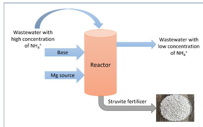
**Figure 3.** Nitrogen recovery by struvite precipitation.
