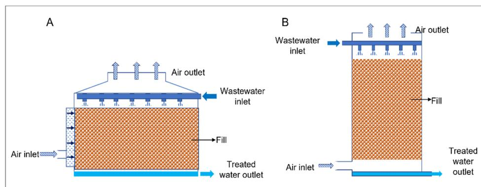
**Figure 4.** (A) Cross-flow and (B) countercurrent ammonia stripping towers.
