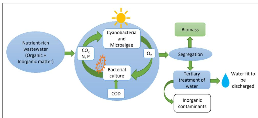
**Figure 2.** Nitrogen recovery from wastewater using microalgae and cyanobacteria.
