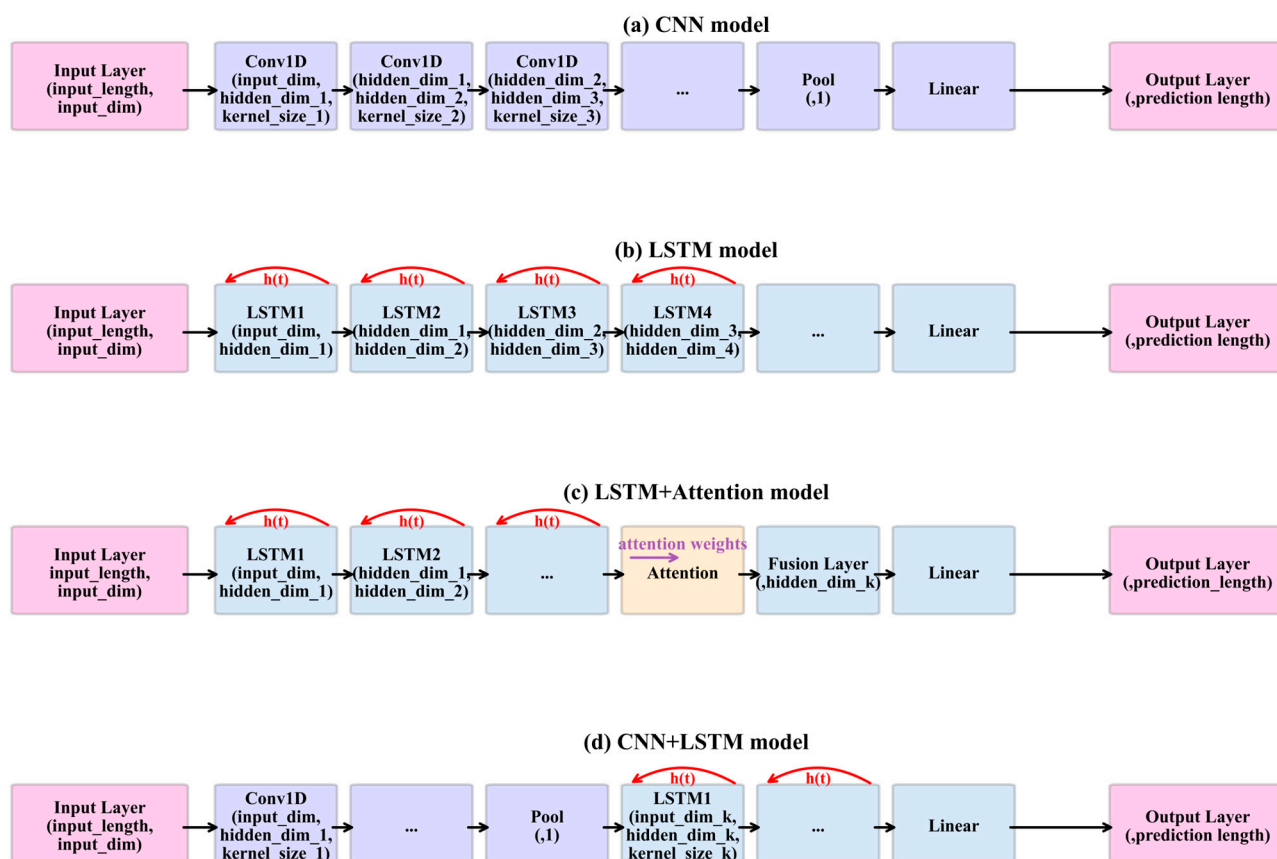
Figure 4. Structure of CNN (a), LSTM (b), LSTM+Attention (c), and CNN+LSTM (d) for one sample. “...” denotes the repetition of the structure of previous modules. The arrows denote the program flow.
