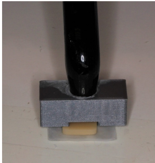
Figure 2. A photo of the jig and light used to conduct the light-curing step of the experiment.
