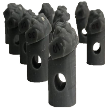
Figure 3. Experimental models with cylindrical base for traction tests.
