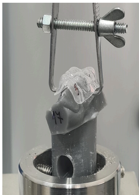
Figure 5. Dislodgement of the aligner using traction equipment.
