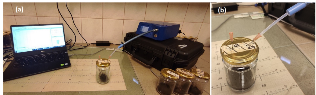
Figure 2. (a)—Measurement setup using PEN3 electronic nose. (b)—Highlighted jar with soil sample during measurement procedure.
