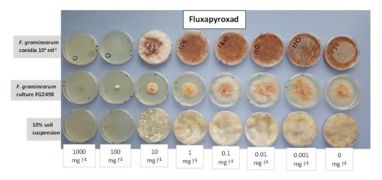
**Figure 1.** Different concentrations of fluxapyroxad added to potato dextrose agar (PDA) and tested for their potential as a selective inhibitor for the development of a selective medium for *Fusarium*
