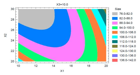
Figure 4. Contour plot for globule size.
