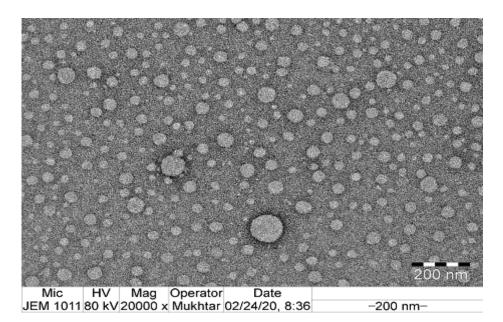
Figure 6. TEM image of the optimized naringenin nanoemulsion.
