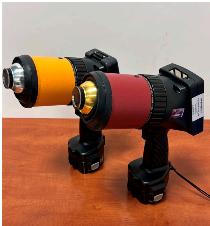
Figure 3. Reflectometer Solar 410 and Emissometer ET-100 (Surface Optics Corporation).
