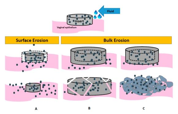
**Figure 2.** Schematic of the different processes of topical insert disintegration with the introduction of vaginal fluid. Surface erosion: (**A**) The size of the insert decreases as the surface disintegrates releasing drug. Bulk erosion: The size of the insert first increases due to fluid uptake and swelling, followed by (**B**) breakdown of the insert into smaller pieces until fully disintegrated or (**C**) transformation from the solid state into a gel.
