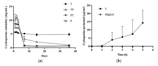
**Figure 3.** (a) Cyclosporine's apparent solubility when incorporated in micelles of TPGS, poloxamer 407, and TPGS:poloxamer 407. (b) Transconjunctival permeation profile of cyclosporine from formulation T (n = 4) and Miglyol<sup>®</sup> solution (drug conc. = 5 mg/mL; n = 3).
