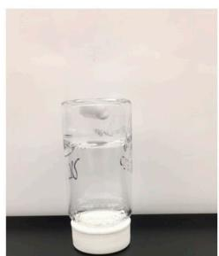
**Figure 1.** Solution of 20% *w/w* poloxamer 407 in water (**A**) at 4 °C prior to heating and (**B**) after heating on a stir plate until gelation occurred, causing the stir bar to stop moving.
