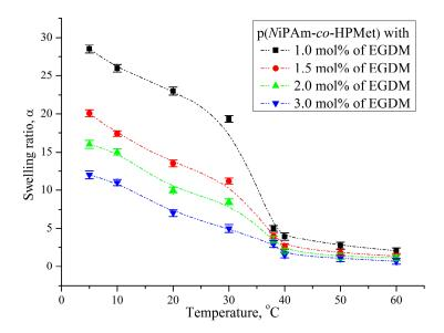
**Figure 2.** Change in the swelling ratio,  $\alpha$ , of p(*N*iPAm-*co*-HPMet) depending on temperature. Error bars represent the standard deviation of three replicates.
