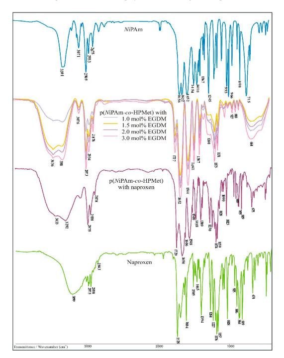
**Figure 3.** FTIR spectra of monomer *NiPAm*, synthesized p(*NiPAm-co*-HPMet) hydrogels with 1.0, 1.5, 2.0 and 3.0 mol% of EGDM, p(*NiPAm-co*-HPMet) hydrogel with 1.0 mol% of EGDM with incorporated naproxen and naproxen.
