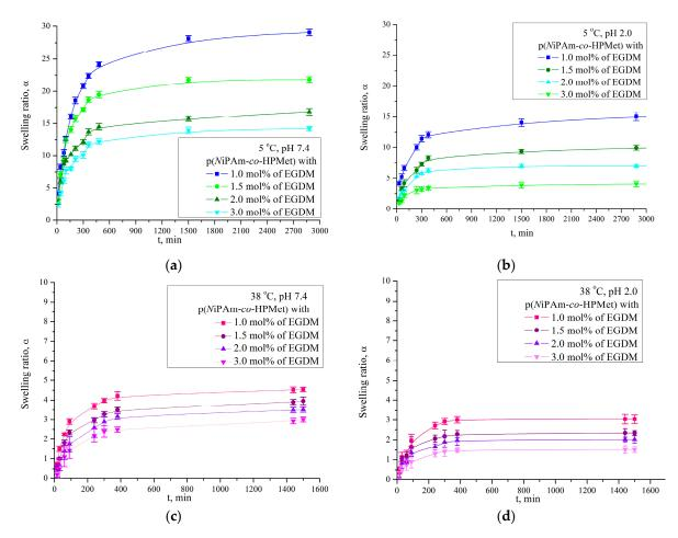
**Figure 1.** Change in the swelling ratio,  $\alpha$ , of p(NiPAm-*co*-HPMet) with 15 mol% HPMet and 1.0; 1.5; 2.0 and 3.0 mol% of EGDM, depending on temperature at: (**a**) 5 °C and pH 7.4; (**b**) 5 °C and pH 2.0, (**c**) 38 °C and pH 2.0; (**d**) 38 °C and pH 2.0. In each figure, error bars represent the standard deviation of three replicates.
