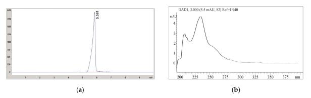
Figure 8. (a) Chromatogram of naproxen from HPLC, (b) UV spectrum from DAD detector.
