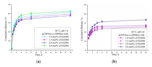
**Figure 9.** In vitro cumulative release of naproxen from p(NiPAm-*co*-HPMet) hydrogels at 38 °C: (**a**) at pH 7.4, (**b**) pH 2.0. In each figure, error bars represent the standard deviation of three replicates.
