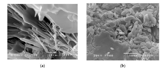
**Figure 6.** SEM micrographs of p(*N*iPAm-*co*-HPMet) sample with 1.0 mol% of EGDM: (**a**) in xerogel state (magnification  $1500 \times$ , scale bar 10 µm) and (**b**) in hydrogel state  $500 \times$  (magnification  $500 \times$ , scale bar 50 µm).
