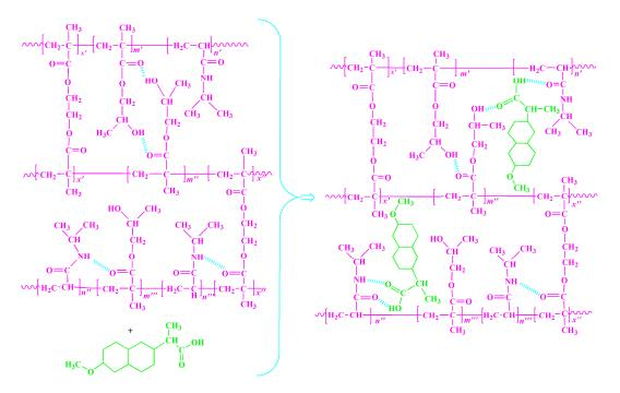
Figure 7. The naproxen incorporation into the p(NiPAm-*co*-HPMet) hydrogels.
