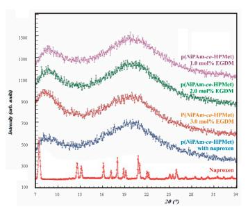
**Figure 4.** XRD diffractograms of: the copolymers p(NiPAm-co-HPMet) with 1.0 mol%, 2.0 mol% and 3.0 mol% of cross-linker EGDM; p(NiPAm-co-HPMet) with 1.0 mol% of EGDM with incorporated naproxen; and naproxen.
