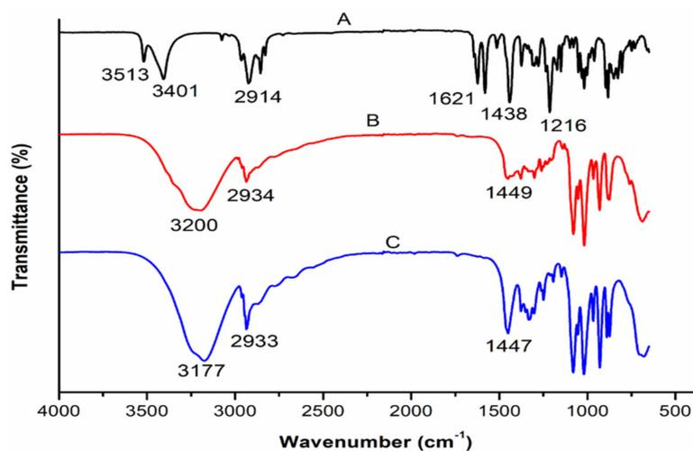
**Figure 4.** FTIR spectra of (A): pristine CBD; (B): CBD-free transfersomes; and (C): optimized CBD-loaded transfersomes (T6).
