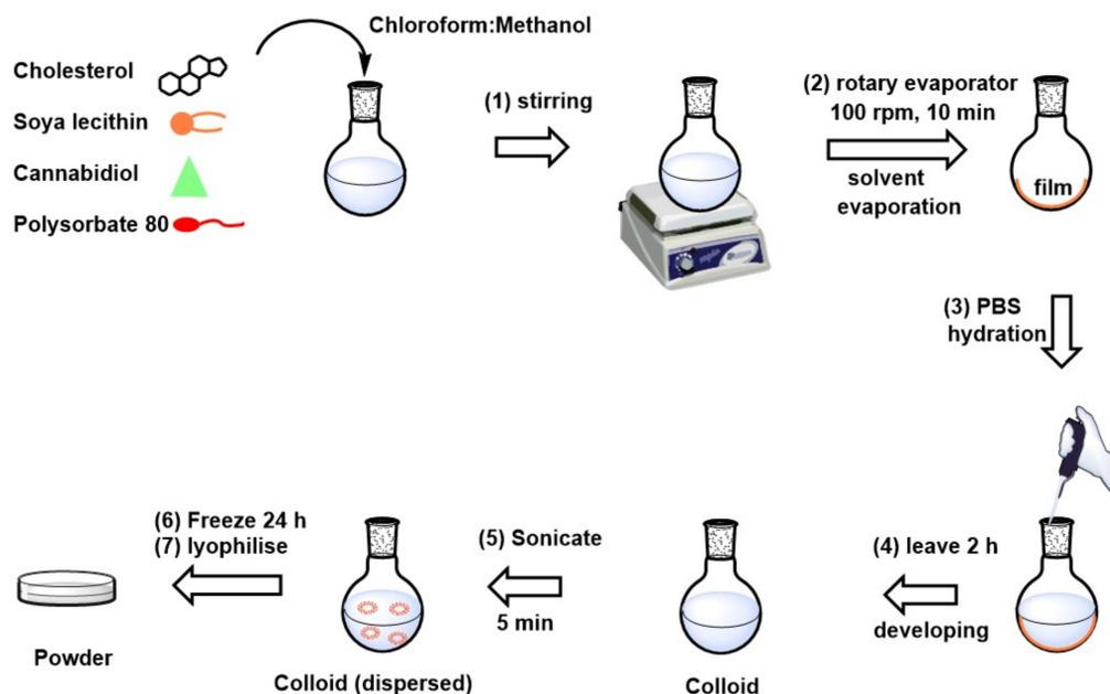
**Figure 1.** Schematic representation of methodology employed for the preparation of CBD-loaded transfersomes.
