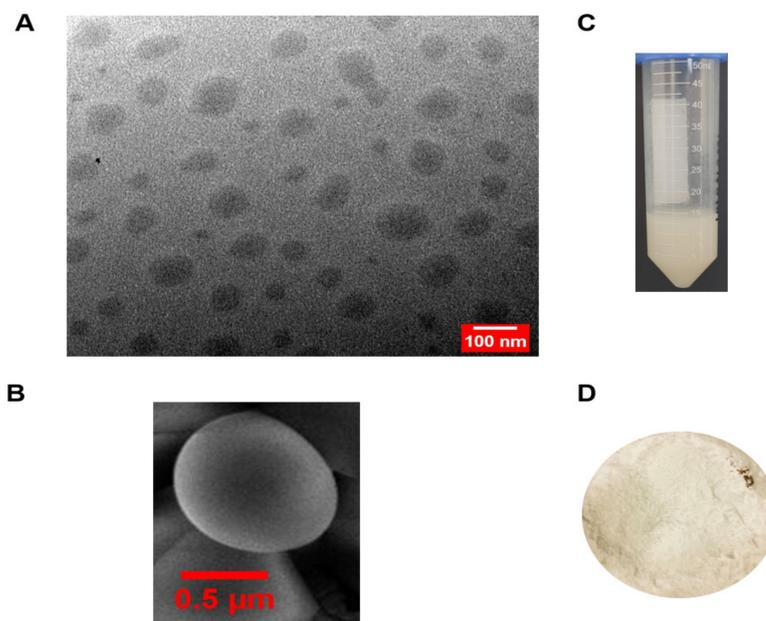
**Figure 2.** Typical macro- and microscopic imagery of the optimized CBD-loaded transfersome formulation (T6). (A) TEM image (scale bar 100 nm); (B) SEM image; (C) physical appearance of the transfersomes (T6); (D) lyophilized free-flowing powder of the transfersomes (T6).
