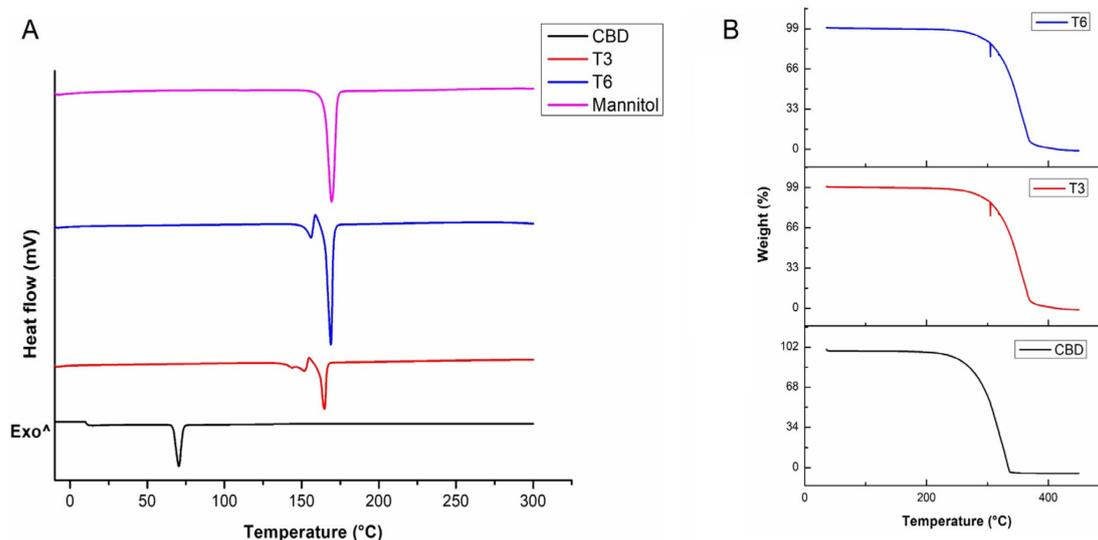
**Figure 3.** (A) DSC thermogram and (B) TGA thermogram of pure CBD, transfersomes (T3) and CBD-loaded transfersomes (T6) respectively.
