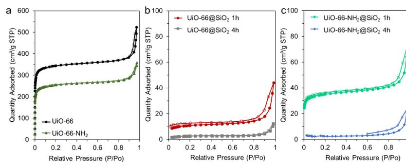
**Figure 5.** Nitrogen adsorption–desorption isotherms measured for UiO-66 and UiO-66-NH<sub>2</sub> (a); UiO-66@SiO<sub>2</sub> 1 h and UiO-66@SiO<sub>2</sub> 4 h (b); UiO-66-NH<sub>2</sub>@SiO<sub>2</sub> 1 h and UiO-66-NH<sub>2</sub>@SiO<sub>2</sub> 4 h (c). Filled markers represent adsorption branches of isotherms, while empty ones designate desorption branches.
