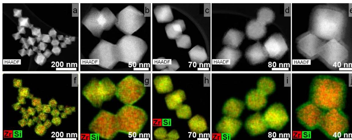
**Figure 2.** HAADF-STEM images and corresponding Zr-Si elemental maps for UiO-66@SiO<sub>2</sub> samples obtained by incubation of PVP-grafted UiO-66 MOFs in TEOS for 0.5 (a,f); 1 (b,g); 2 (c,h); 4 (d,i); 24 h (e,j).
