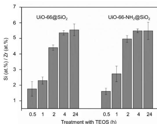
**Figure 3.** Si/Zr ratio in UiO-66@SiO<sub>2</sub> and UiO-66-NH<sub>2</sub>@SiO<sub>2</sub> MOFs treated with TEOS for different durations.
