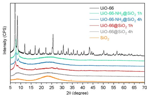
**Figure 4.** XRD patterns collected for intact UiO-66 nanoparticles, SiO<sub>2</sub> nanoparticles, and TEOS-treated UiO-66@SiO<sub>2</sub> and UiO-66-NH<sub>2</sub>@SiO<sub>2</sub> samples.
