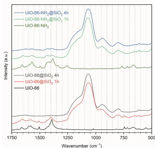
**Figure 6.** ATR-FTIR spectra collected for intact UiO-66 and UiO-66-NH<sub>2</sub> nanoparticles compared to UiO-66@SiO<sub>2</sub> and UiO-66-NH<sub>2</sub>@SiO<sub>2</sub> MOFs treated with TEOS for different durations.
