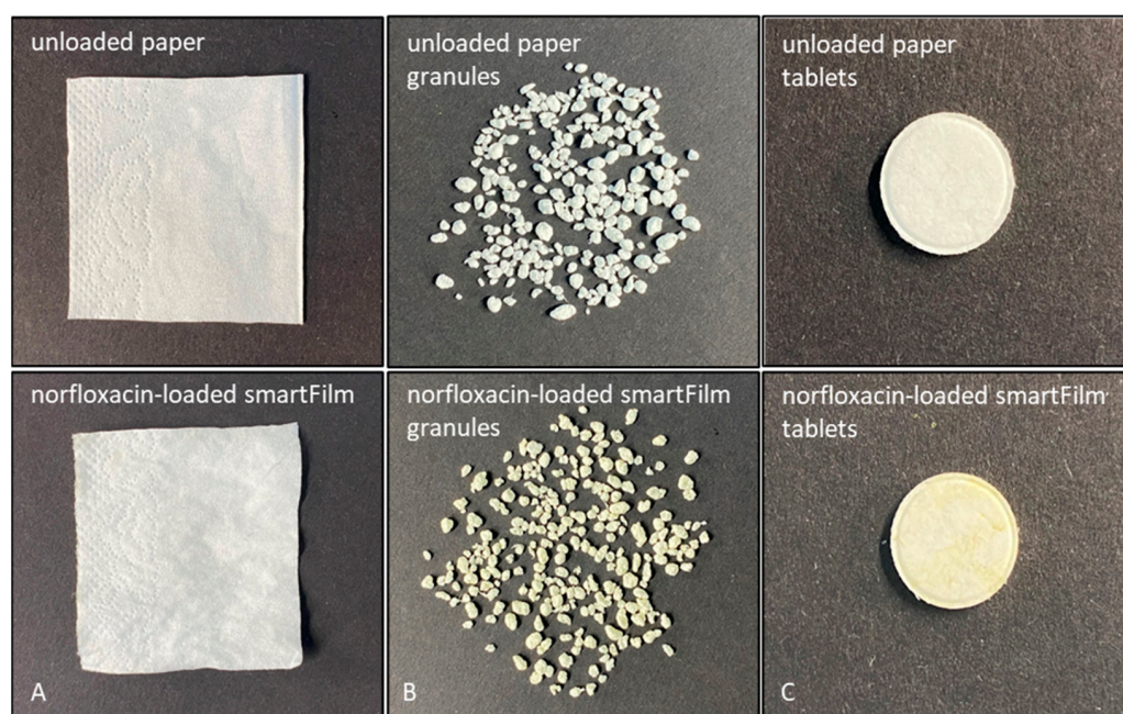
Figure 2. Macroscopic images of (A): unloaded paper (upper) and paper loaded with norfloxacin (smartFilms, lower), (B): unloaded paper granules (upper) and norfloxacin-loaded smartFilm granules (lower) (C): unloaded paper tablets (upper) and norfloxacin-loaded smartFilm tablets (lower).
